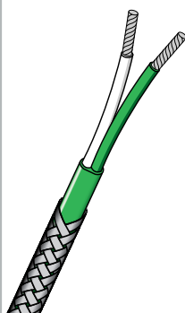
Stainless Steel Braided PFA Flat Twin One pair of stranded conductors. Cores PFA insulated. Pair laid flat. PFA sheathed. Stainless steel braided overall.
