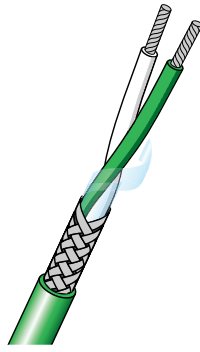
Flame Retardant Silicone Rubber, Twisted Pair with Nickel Plated Copper Braid One pair of stranded conductors. Cores Silicone Rubber insulated. Pair twisted and Mylar® taped with nickel plated copper braid. Silicone Rubber sheathed.
