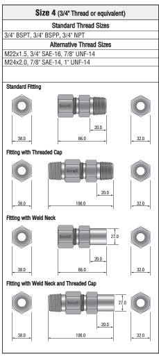
Please note: The overall length will vary slightly depending on the sealant used and the tube size.
