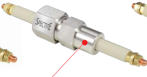
Weld Neck Supplied without thread for permanent installation into the process by welding. Specify as 'WELD' for the thread size in the order code.
