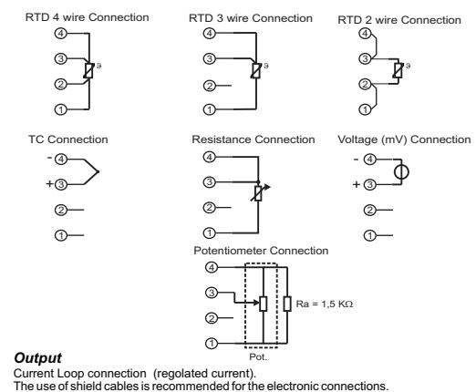
Current Loop connection (regulated current). The use of shield cables is recommended for the electronic connections.
